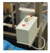
The Mach-2P case packer can be started from (two) locations (optional.) An HMI control panel is integral to the machine guarding and there is also a remote push button station.
