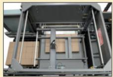
The row sweep pushes each row onto the elevator, forming a layer one row at a time. The elevator then positions the layer over the top of the load, extends and places the layer on the load.
