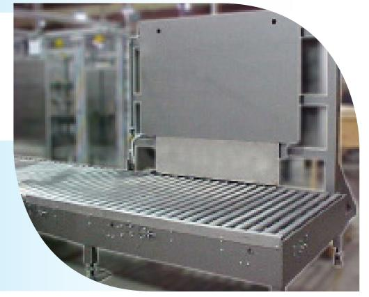
Station 1: Roller Conveyor – Nip roller pulls the slipsheet from underneath the bundles and moves two bundles to Station 2 while leaving two bundles at Station 1.
