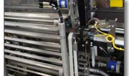
**Right:** Walk-in design allows easy access into machine for cleaning & maintenance.
