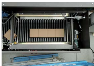
B. Cases convey into the row forming area where each layer is formed one row at a time.
