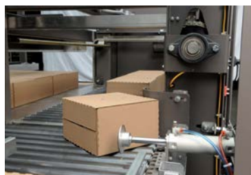
A. Cases enter an LL Series Palletizer where the case/tray turner and case stops help form the desired row pattern.
