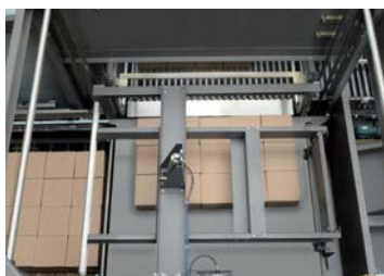
C. The row sweep pushes each row onto the elevator, forming a layer one row at a time. The elevator then positions the layer over the top of the load, extends and places the layer on the load.
