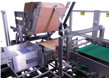
B. MAGAZINE A single case blank is picked from the magazine and the case is set into the loading station.
