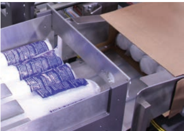
C. CASE LOAD The major flaps are contained so the case remains in the loading section and the loading funnels open the minor flaps and the case is loaded.
