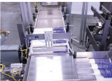
A. PRODUCT INFEEED Flexible package conveys onto staging conveyor or racetrack (optional) to build appropriate pack patterns
